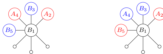
Fig. 6. CFON k -coloring game on a star graph S_{n-1} : Bob starts coloring the central vertex, the first two colors are duplicated in the next four turns ((left) A_2, A_4 are red and B_3, B_5 are blue, (right) A_2, B_5 are red and B_3, A_4 are blue).
