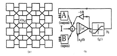
Figure 1: Cellular Neural Networks:(a) Array Structure and (b) Block Diagram
