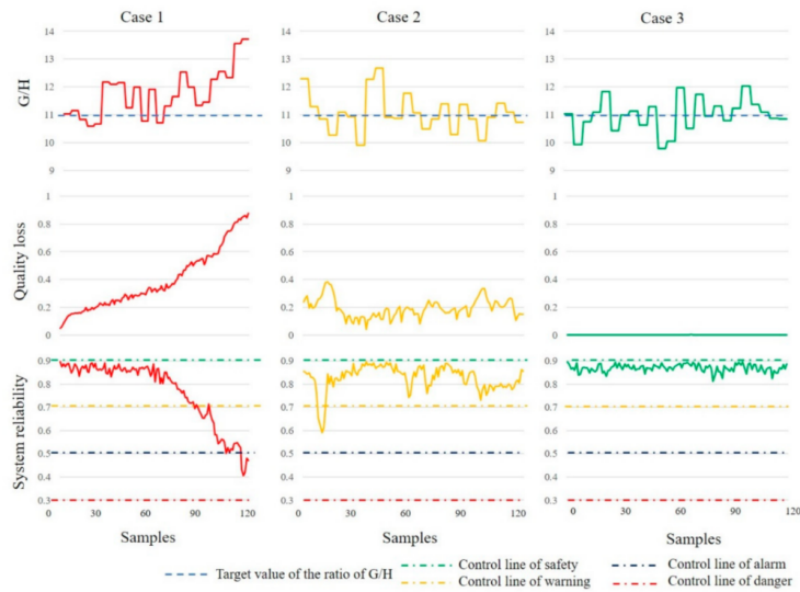
Fig. 4. Comparison of reliability estimation results for the R-22 reactor operating unit.
