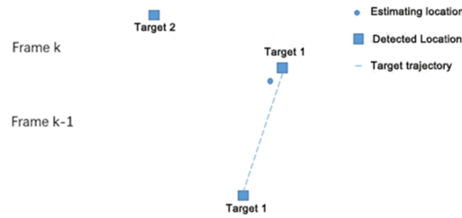
Fig. 9. Schematic of target association
