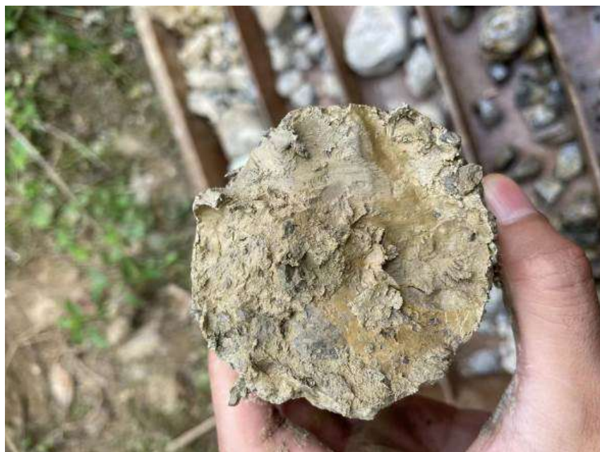
Fig. 5. Mirror and scratch characteristics of ZK03
