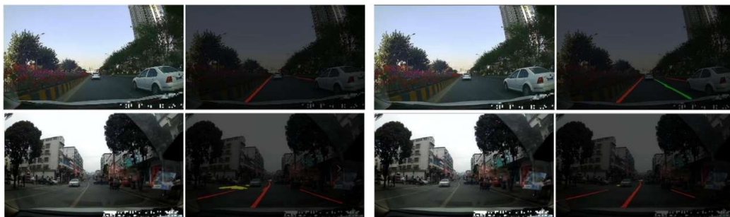
Fig. 9. The In comparison to the prediction outcomes of the standard U-Net network enhanced with the SE attention module, the inference results of the standard U-Net network are presented on the left, while those incorporating the SE attention module are illustrated in the image on the right
